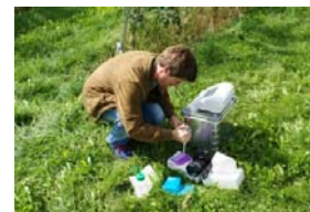
Fig. 2: LAMP portable device (Genie II, Optigene Ltd.) working on battery was taken out of the laboratory for a field trial experiment where results could directly be visualized on the screen of the machine within 20 min..
